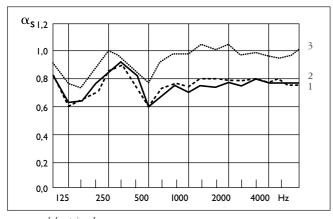
$\alpha_s = soundabsorption degree:$ an absorption of 1.0 indicates a 100% absorption of sound.
